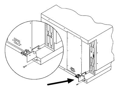
2. Ensure that the rack's anti-tip rails are extended.
